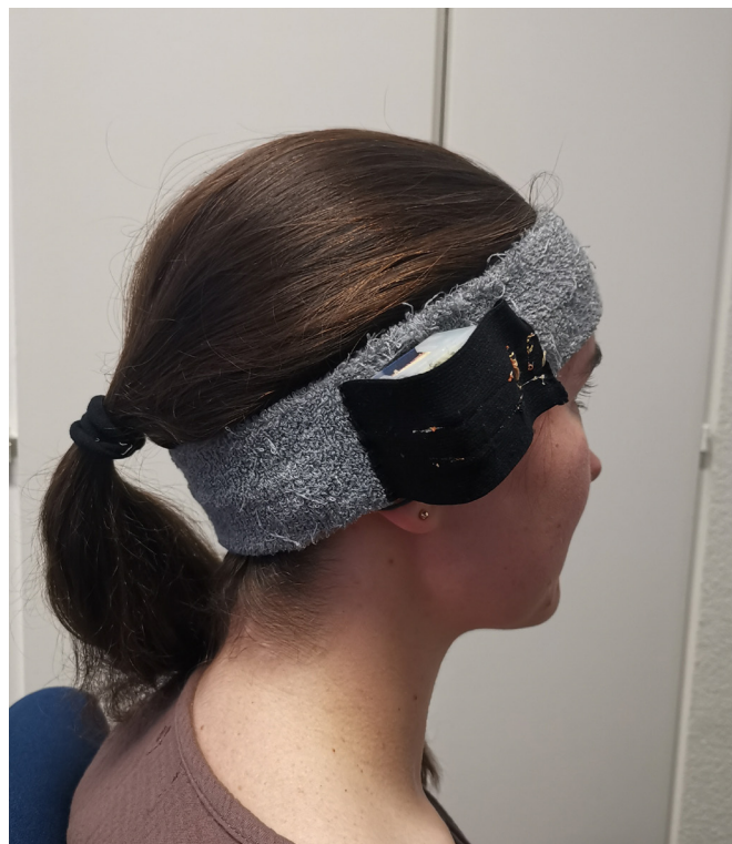
Figure 2 The Auracle: eating recognition system.
