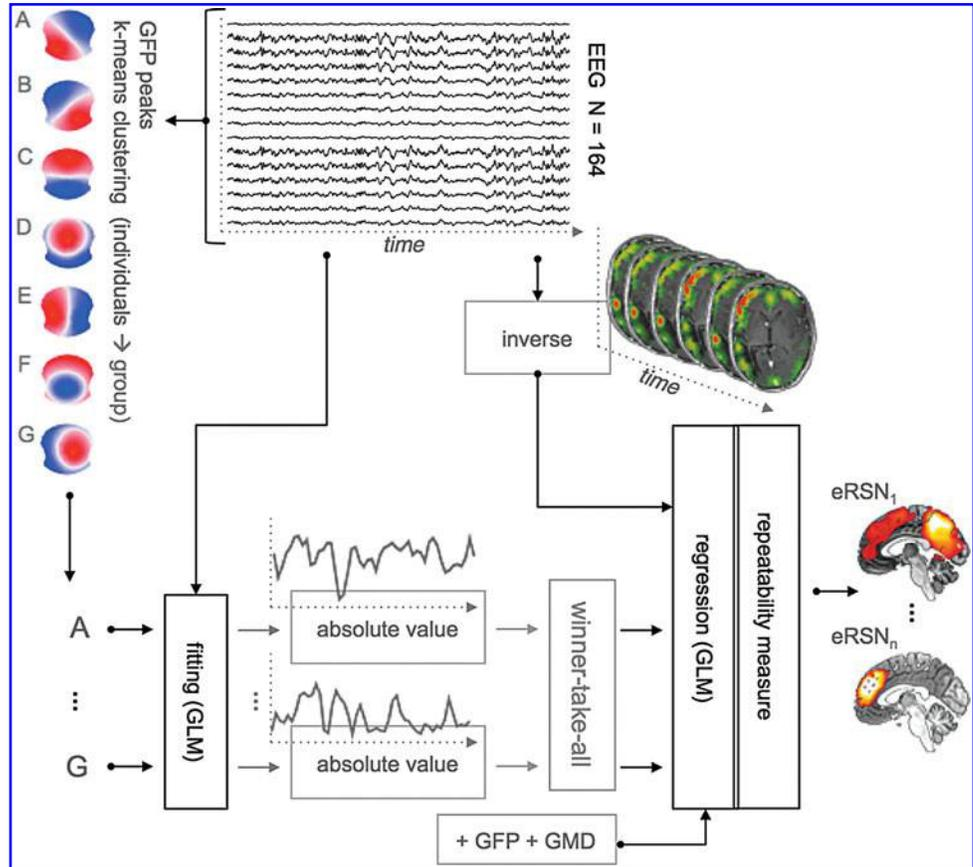
The GFP regressor helps eliminate the bias induced by the signal power fluctuations; the GMD regressor can diminish the contributions of the moments of transitions between states, when the SNR is very low and the signal association to a particular state is weak (Lehmann and Skrandies, 1980). Similarly to an fMRI GLM-based analysis, the result of this process is a beta variable distribution associating “activity” to voxels matching a certain temporal pattern.
