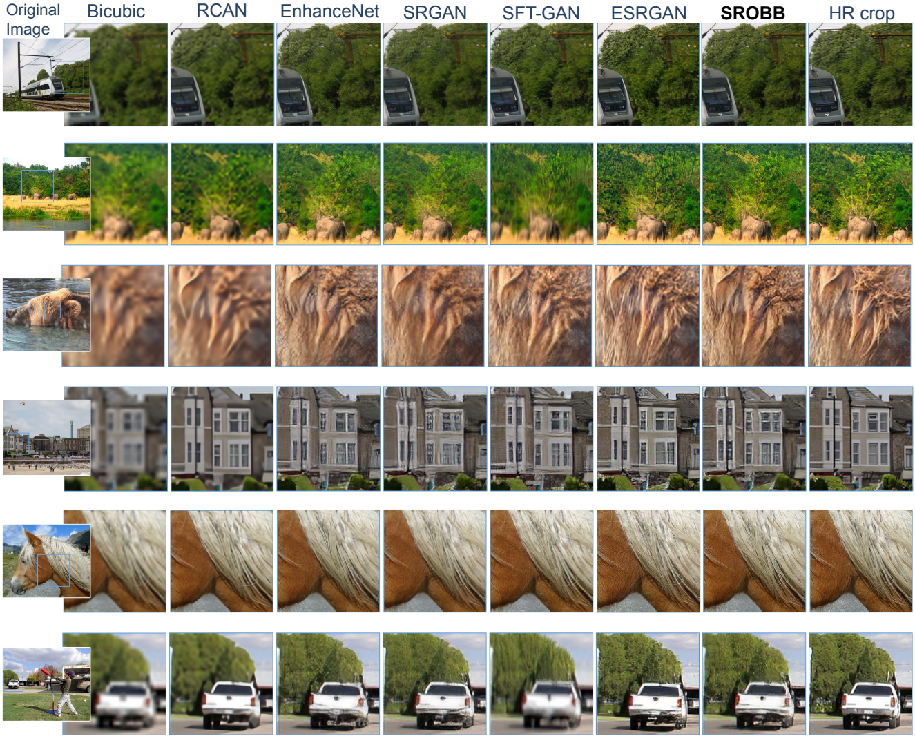
Figure 6. Qualitative results on a subset of the COCO-Stuff dataset [4] images. Cropped regions are zoomed in with a factor of 2 to 5 to have a better comparison. Results from left to right: bicubic, RCAN [44], EnhanceNet [27], SRGAN [20], SFT-GAN [35], ESRGAN [36], SROBB (ours) and a high resolution image. Zoom in for the best view.
