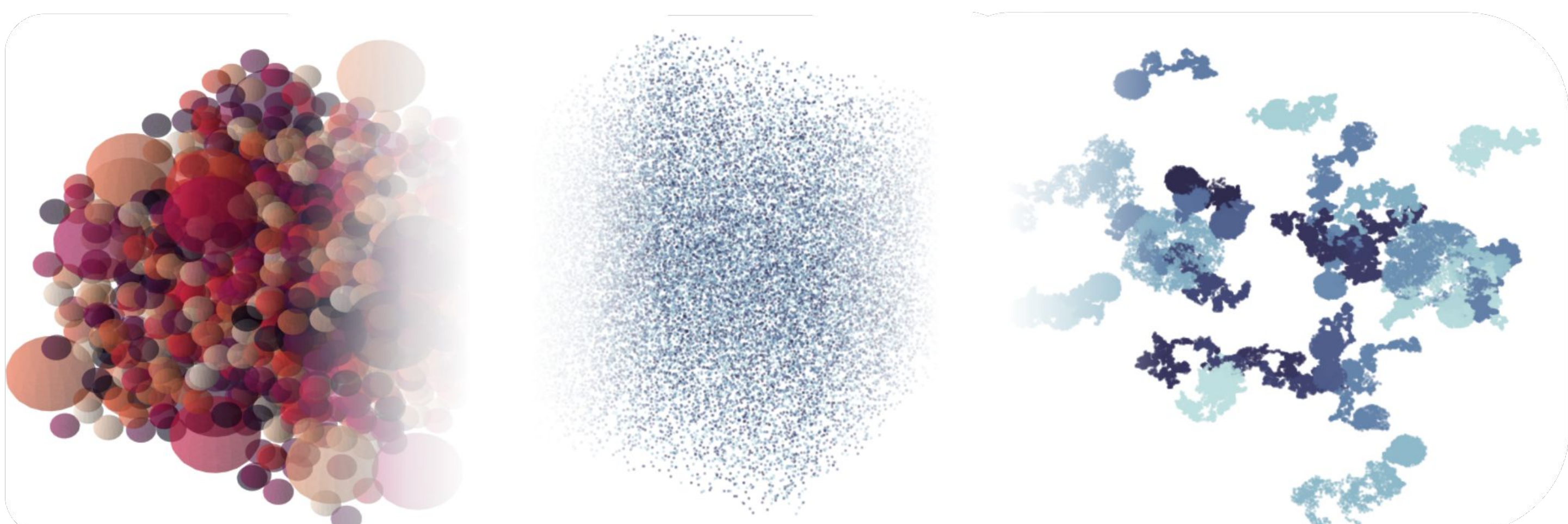
Monte-Carlo simulations: Substrate (left), particles initialization (centre) and trajectories (right)
