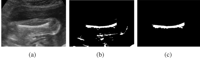
Fig. 10. Entropy-based segmentation method. (a) Original image. (b) Result after entropy-based segmentation. (c) Final selected femur.
