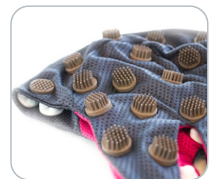
Dry EEG electrode caps NES Lab, CHUV - Lausanne
