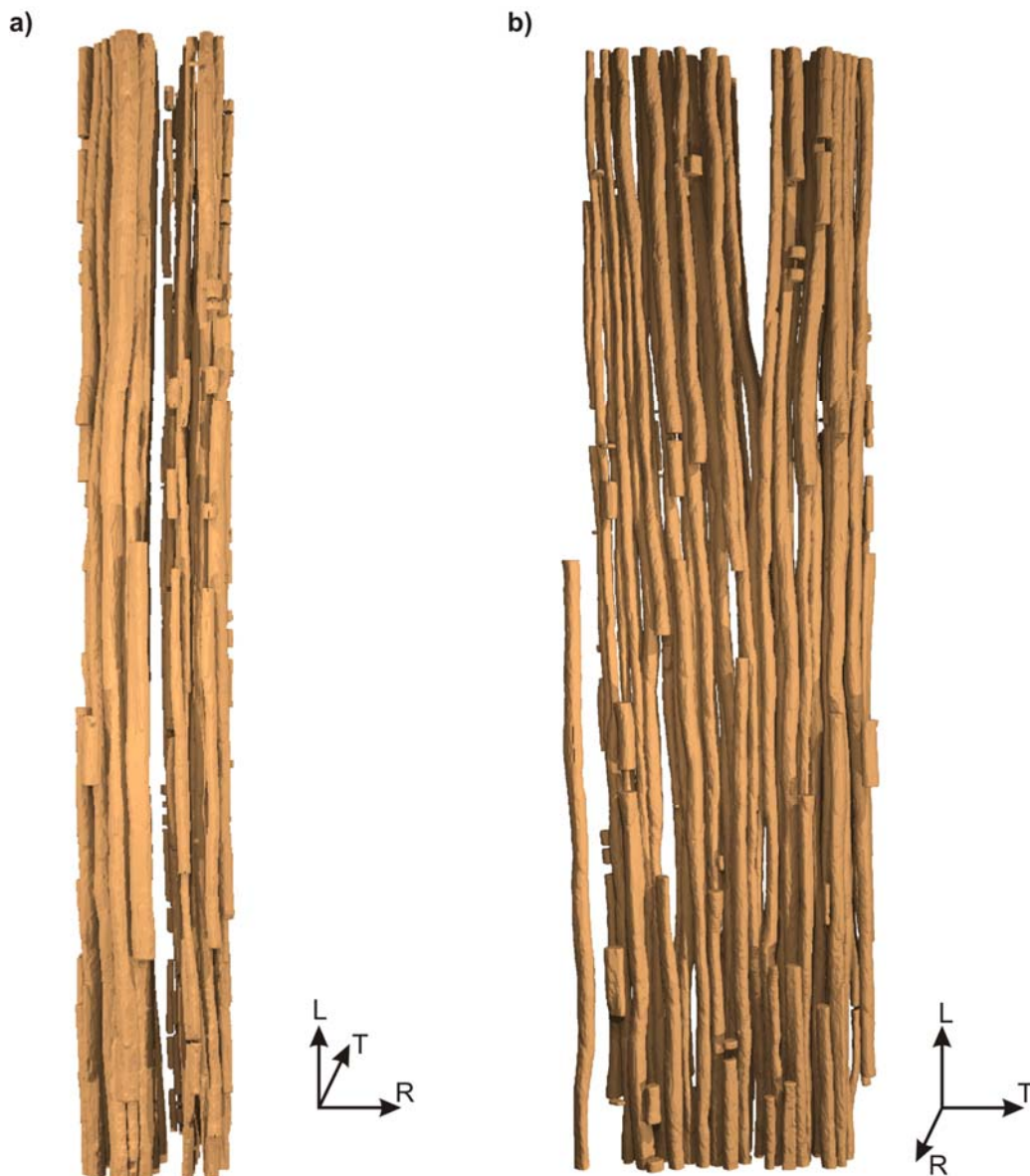
Figure 3 Vessel network of beech wood looking along T-direction (a) and R-direction (b). Sample height is 3 mm. Note that the displayed vessel discontinuities are mainly due to vessels moving in and out of the extracted volume.
