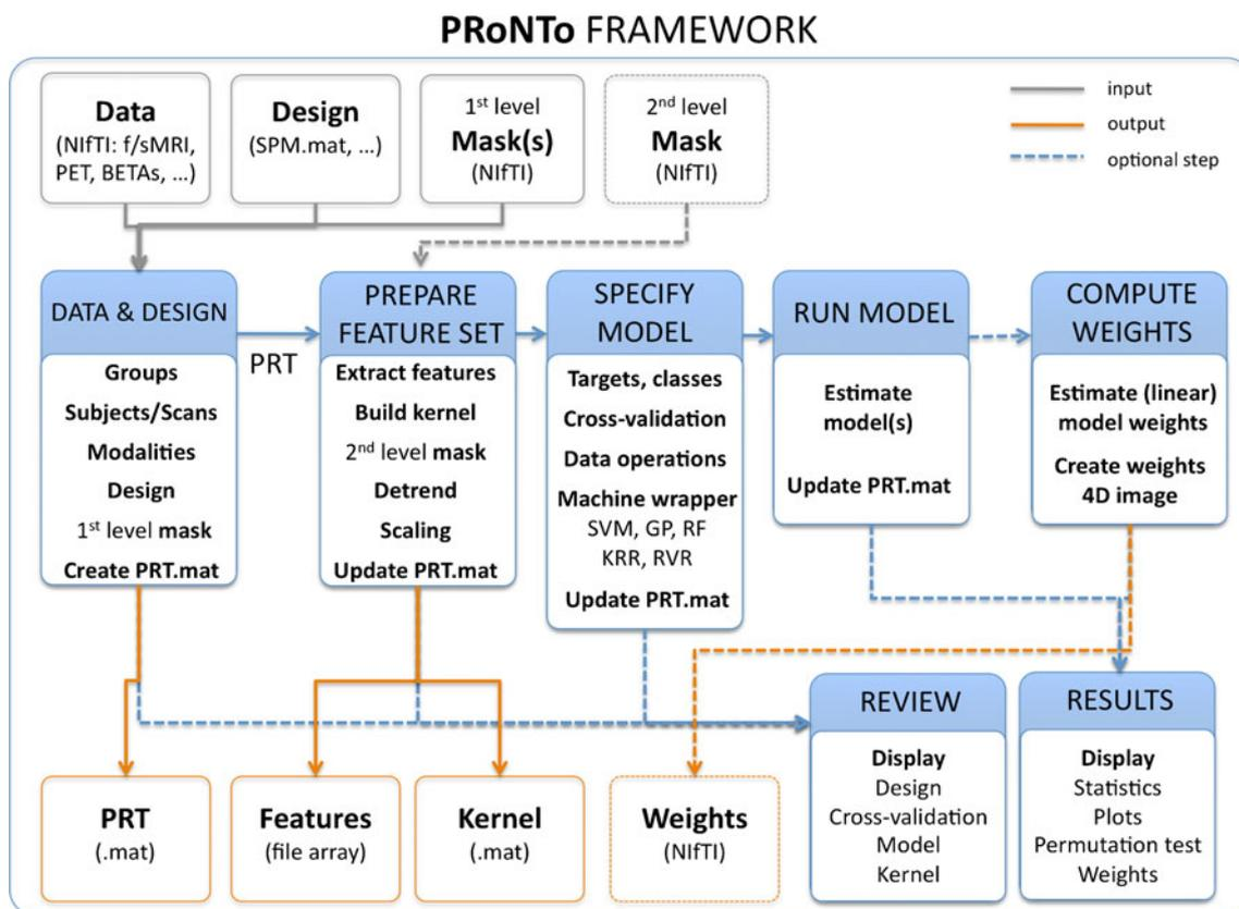
**Fig. 1** PRoNTTo framework. PRoNTTo has five main analysis modules (blue boxes in the centre): dataset specification, feature set selection, model specification, model estimation and weights computation. In addition, it provides two main reviewing and displaying facilities (model, kernel and cross-validation displays, as well as, results display). PRoNTTo receives as input any NIfTI images (comprising the data and a first-level mask, while an optional second-level mask can
