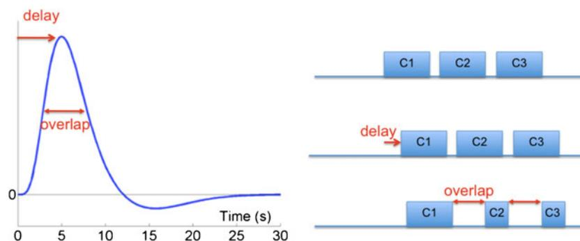
**Fig. 5** HRF correction. On the left is the standard HRF response. On the right is the effect of the delay and overlap on the number of independent scans (C1, C2 and C3 correspond to three different experimental conditions and the blue boxes correspond to various scans acquired during each condition). In fMRI datasets, the nature of the
