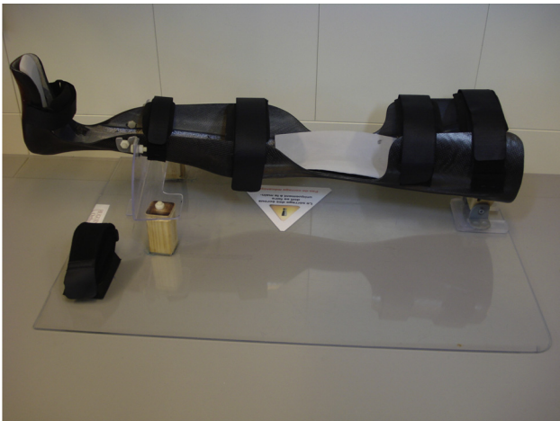
Fig. 2 – The stabilizing system of the knee for MRI acquisitions.
