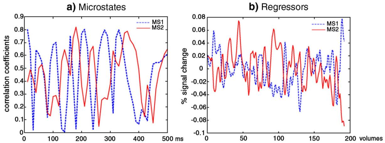
**Fig. 2.** Scale invariance in the time course of EEG and fMRI signals. a) Time course of the spatial correlation coefficients of MS1 and MS2 in a randomly chosen time interval of 500 ms for one subject; the signals are strongly anti-correlated. b) Time course of the EEG signal after convolution with the HRF for all 200 TRs; the same anti-correlation of time courses is preserved after the convolution, i.e. temporal low-pass filtering.
