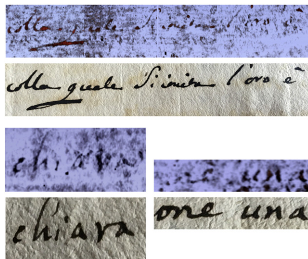
Fig. 6. Several examples of tomography reconstructed inner page portions revealing words and sentences (top), compared to visible pictures (bottom).
