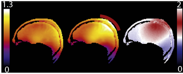
Fig. 1. Example of improved local transmit B_1^+ field in the motor cortex using a dielectric pad containing a solution of deuterated water and barium titanate (dielectric permittivity of 160) (red bar in the middle image). Experimental B_1^+ field maps without (left) and with (middle) the dielectric pad present. The ratio of the two images (right) shows a B_1^+ increase by a factor of two in the motor cortex, above which the pad was placed. The scale of the B_1^+ maps, obtained using the SAZRAGE (SAaturation-prepared with 2 Rapid Gradient Echoes) sequence [71] ( TR = 2400 ms, TE = 0.78 ms, TD_1 = 45 ms, TD_2 = 1800 ms, \alpha_1 = 4^\circ , \alpha_2 = 10^\circ , 2 \times 2 \times 2.5 mm 3 resolution and a 128 \times 128 \times 64 matrix size acquired with sagittal orientation, TA = 1 min 55 s, reference voltage = 170 V) corresponds to a multiplicative factor of a desired flip angle (Adapted from Ref. [17], with permission from Elsevier).
