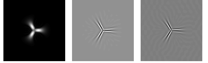
Fig. 3. Three-fold-symmetric wavelet designed by the energy functional in the Fourier domain and visualized in the space domain. From left to right: magnitude, real, and imaginary parts, respectively. Harmonics: S = \{3n : n = 0, \dots, 9\} .
